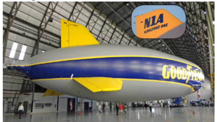
The FAA required Wingfoot One , a Zeppelin model type LZ N07-101, to undergo a complete certification as they considered it a new type of airship. All current and previous built Zeppelin's are model type LZ N07-100s. On August 28, 5 days after Goodyear christened the airship, the FAA approved the national registration number of N1A. Goodyear affixed the N1A registration number to the upper & lower stabilizer-rudders, replacing the German registration of D-LZGY & tri color flag. (AIP Photo)
