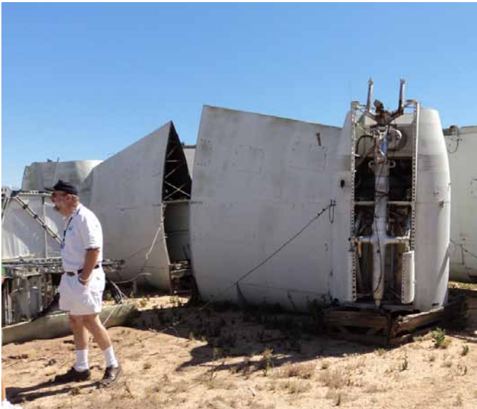
With engine access through the ballonnet ducts, the pylons housed the more substantial 3W main gear and the same radials as the Super Connie.
