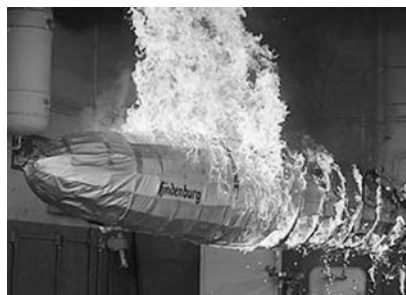
Ed. Caption: Mythbusters model set alight before hydrogen was injected into its interior from a welder's K-bottle. New York Times photo thanks to Walter Lion.
