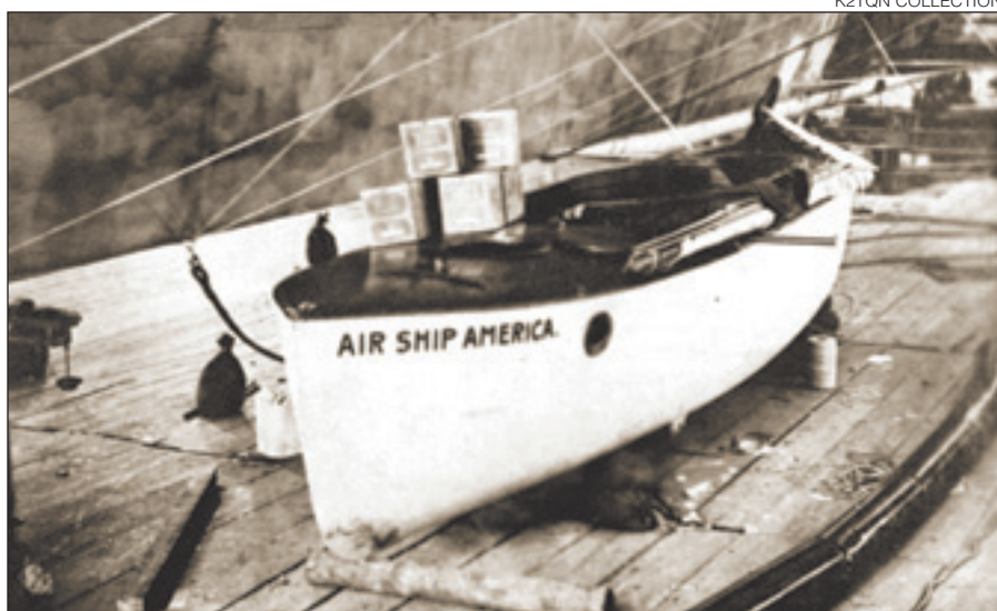
America's lifeboat being prepared for the Atlantic crossing. Jack Irwin's "shack" was located amidships in the lifeboat; from there he would operate a spark transmitter directly under a huge bag of hydrogen gas.
